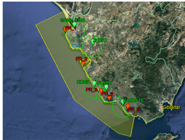
Figure 3: Radar sensor network deployment in the radar scenario: AoI (yellow area), IoOs emplacement and radiation pattern near to the AoI (green) and PR along the coastal border (red).
