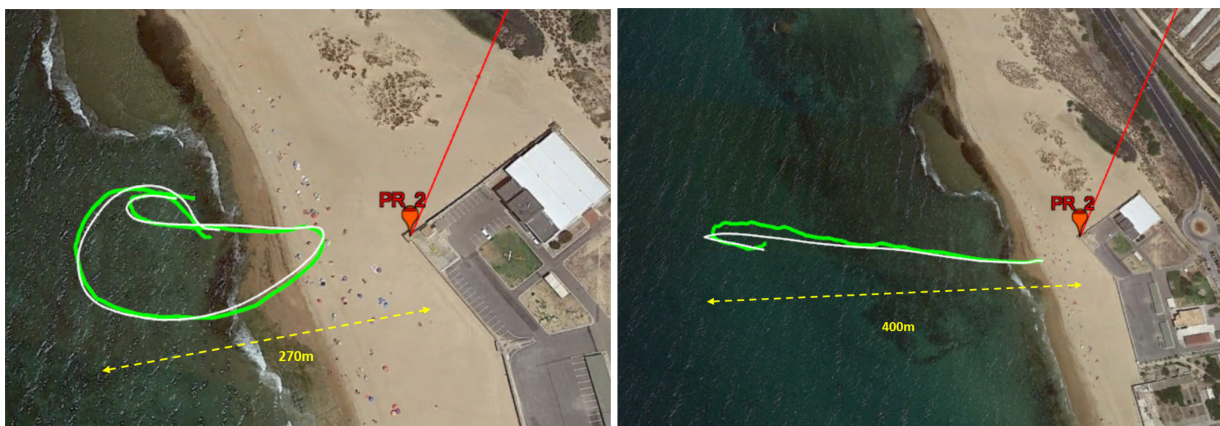
Figure 9: Tracking results for a cooperative DJI Phantom III (green line) and the real target trajectory from the GPS data (white) for two different flying tests.
